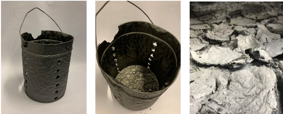
Figure 5: Inside and Outside View of the 30-liter Drum after Pyrohydrolysis Test as well as dust remains in the Trip Tray
