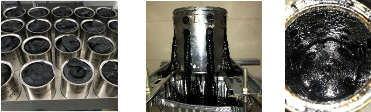
Figure 2: Filled Canister, Drain of the Bitumen and Canister with Remains after Draining
